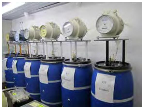
*Complete set up of the 6 LSR, The two (on the left site of the photo) were for air injection. The two in the middle were for H<sub>2</sub>O<sub>2</sub> injection and the two last were the controls with anaerobic conditions*
