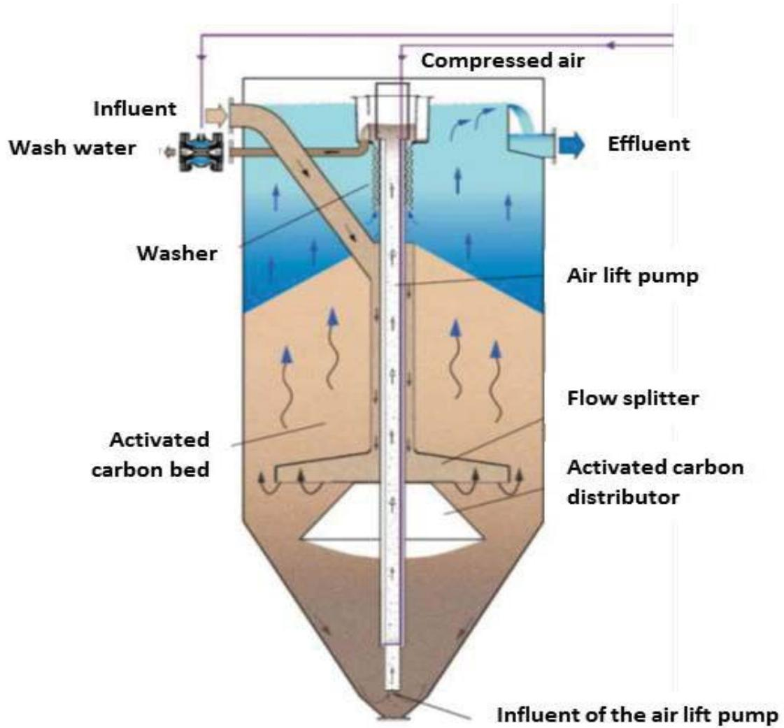
Figure: Schematic of a continuously backwashed filter
