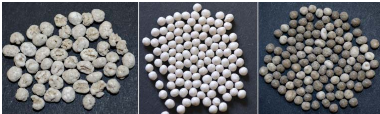
Figure: MAP pellets produced from LFKW wastewater (left), industrial wastewater (middle) and pretreated- sludge filtrate (right)
