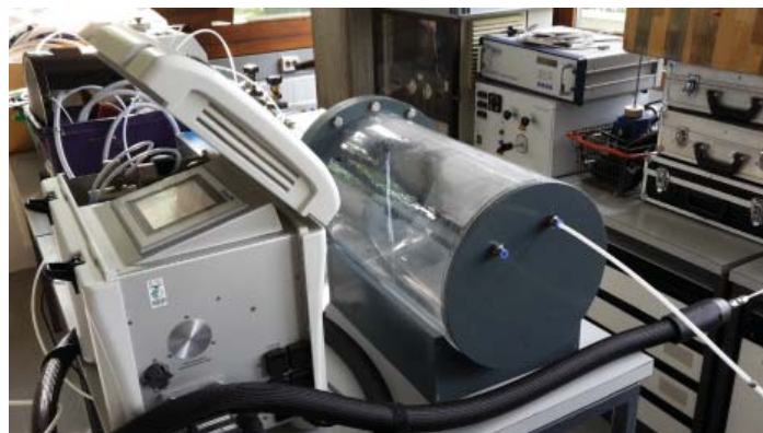
Figure: Measuring cylinder for comparison measurement with dry and humid sample gas
