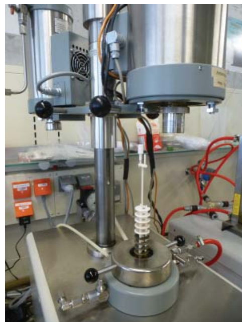
Figure: Thermogravimetric analysis und Helium gas pycnometer
