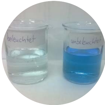
Figure: Samples with methylene blue solutions before (right side) and after (left side) photocatalytic treatment
