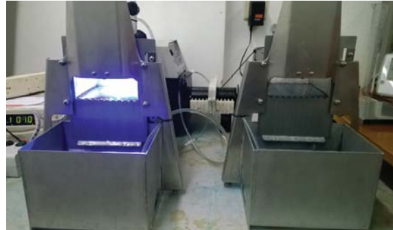
Figure: Experimental setup for photocatalyst testing
