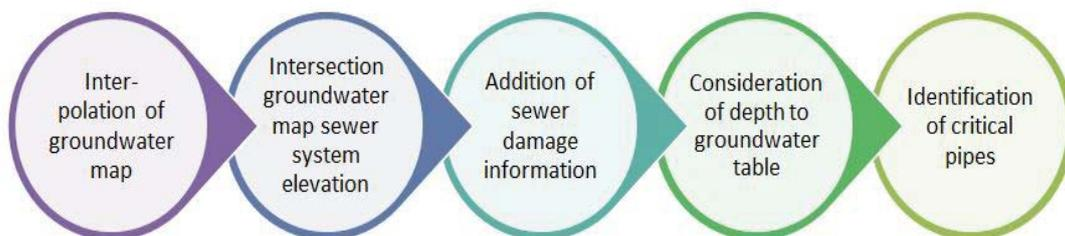
Figure 3: Process flow GIS-methodology for identification of sewer pipes which could cause a critical rise of groundwater level in consequence of sewer system rehabilitation (Bachmann et al. 2015b)
