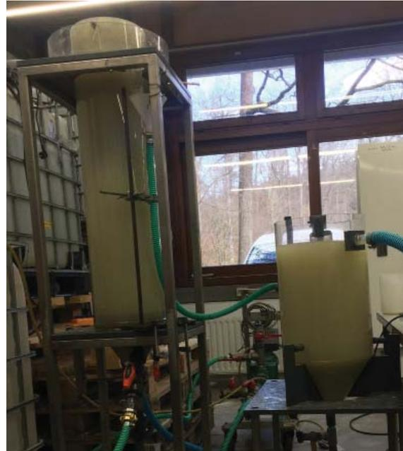
Figure.: Contact reactor for ammonium removal from waste water
